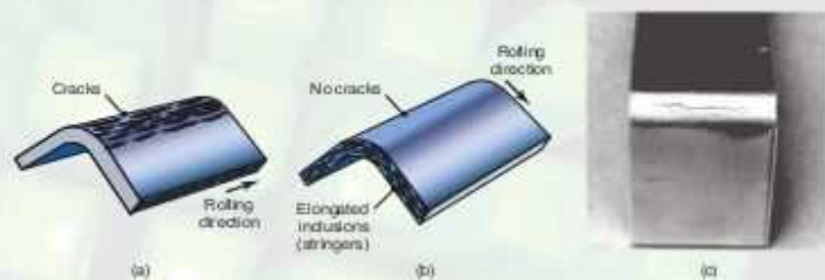
FIGURE 7.17 (a) and (b) The effect of elongated inclusions (stringers) on cracking in sheets as a function of the direction of bending with respect to the original rolling direction. This example shows the importance of orienting parts cut from sheet to maximize bendability. (c) Cracks on the outer radius of an aluminum strip bent to an angle of 90°; compare this part with that shown in (a).
