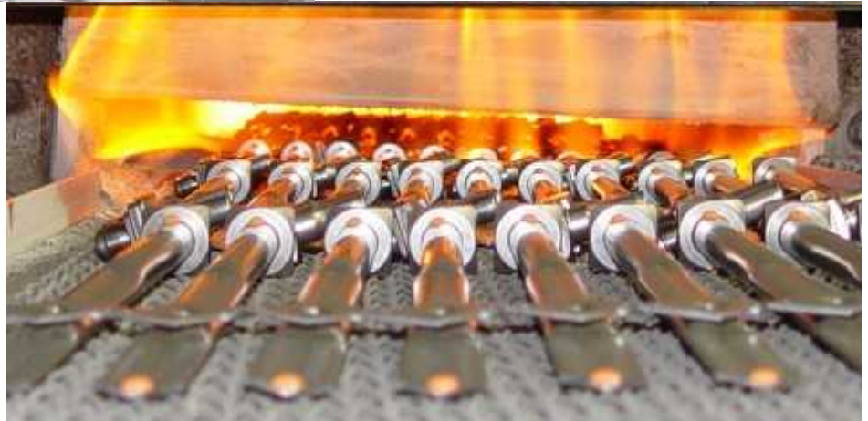
Temperature logging system enters furnace with the product
